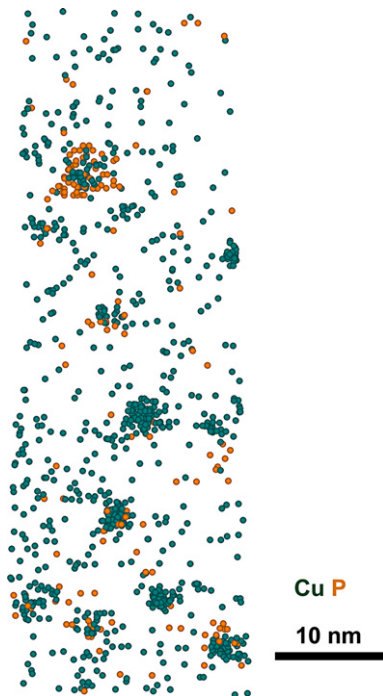
Fig. 8. Atom map from the KS-01 weld that was neutron irradiated to a fluence of 0.8 \times 10^{23} \text{ n m}^{-2} ( E > 1 \text{ MeV} ) at a temperature of 288 \text{ }^\circ\text{C} showing phosphorus segregation to the copper-enriched precipitates and a phosphorus cluster.
